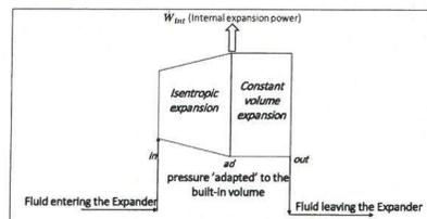
Internal expansion power (W),  $\dot{W}_{int} = \dot{m}_{fluid}(h_{in} - h_{out,s})$ ;
