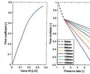
Figure 2. Default flow coefficient to the left and flow multiplier to the right
