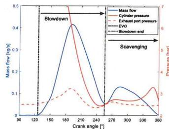
Figure 1. Blowdown portion of the exhaust emptying process.
