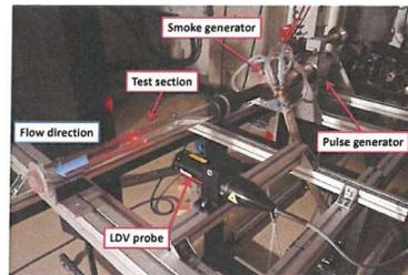
First attempt on Laser Doppler Velocimetry measurement downstream of current pulse generator (February 2019)
