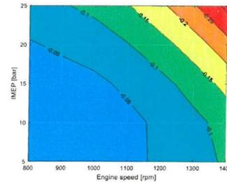
Figure 3. Flow multiplier model effect on pumping work
