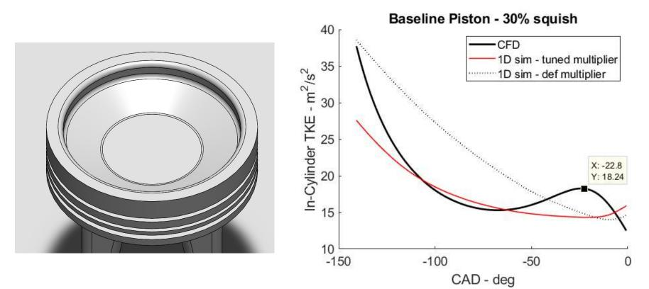
TKE with respect to CAD will be imposed in GT power for modelling piston shapes
