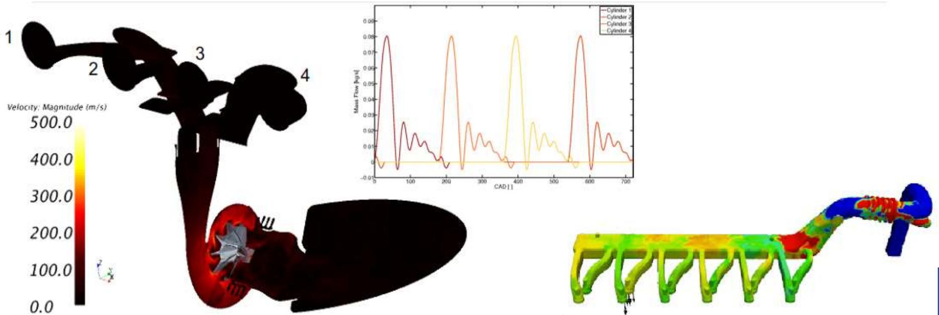
Pulsating flow in an exhaust manifold (VOLVO Cars) integrated with turbine for accurate turbo performance assessment
