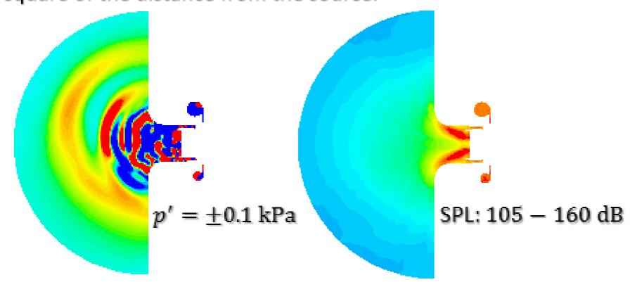
Phase angle evolution of the flow perturbation at off-design operating condition. The figure shows circulating vortical structures upstream and downstream of the impeller, which have been identified as rotating stall. This is observed as a high amplitude noise source.
