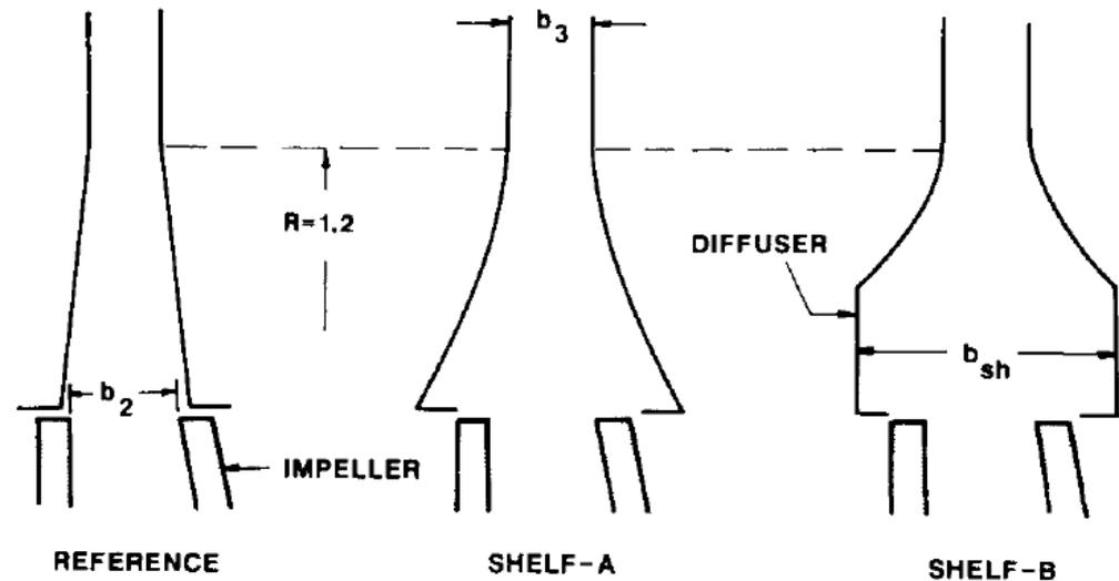
Fig. from G. J. HANUS, Characteristics of a Centrifugal Compressor With a Radial Shelf Diffuser, ASME 87-GT-192
