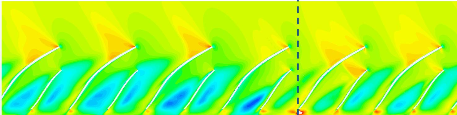
Flush volute overall accelerated throughflow. Visible at VLD inlet. Less symmetrical loading on impeller.
