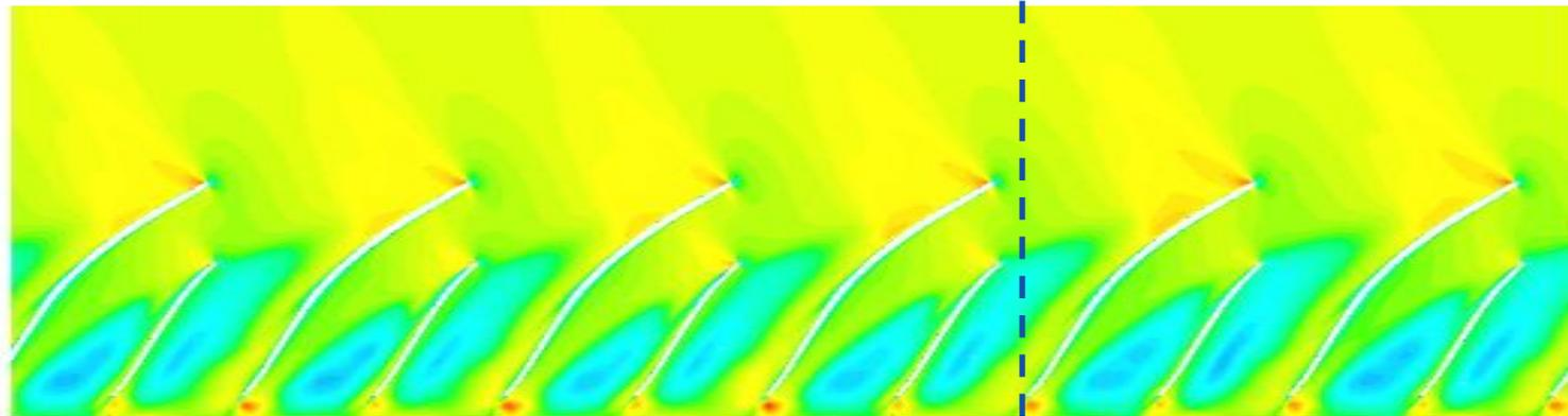
Symmetrically shelved VLD leads to significantly decelerated throughflow. The passage loading is largely symmetrical
