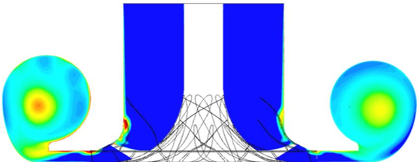
The losses associated with the VLD interaction can be eliminated but reacceleration inside the scroll will impact efficiency at high flow conditions.
