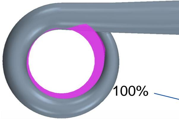
*The baseline volute (right) is modified by trimming the protruding part of the VLD by various percentage. The flush volute (left) has the VLD fully trimmed.*
