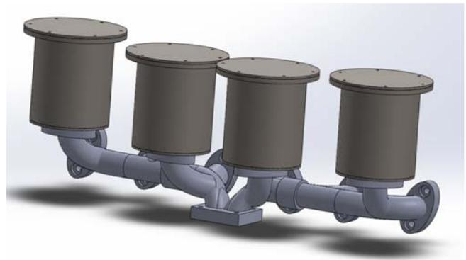
Figure 2. Exhaust manifold with four cylindrical volumes added.
