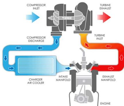
Figure 1. Schematic drawing of turbocharged internal combustion engine.
