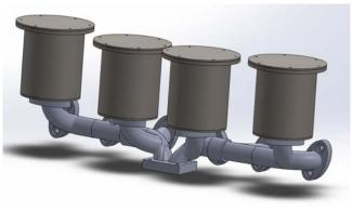
Figure 2. Exhaust manifold with four cylindrical volumes added.
