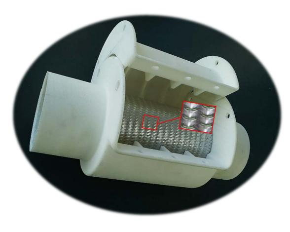
The prototype of compact silencer consisting of straight flow channel made of microperforated panel (MPP), and adjoining cavity. Such compact silencer concept can provide a very high level of sound dissipation.
