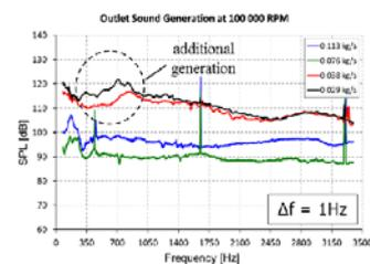
The sound pressure level (SPL) spectrum of generated sound in the outlet branch of the compressor at constant rotor frequency. The mass flow is varied from maximum to minimum i.e. near surge operation.
