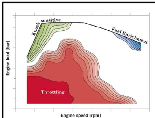
Limits of SI engine efficiency – Gasoline
