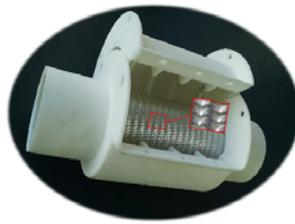
The prototype of compact silencer consisting of straight flow channel made of micro-perforated panel (MPP), and adjoining cavity. Such compact silencer concept can provide a very high level of sound dissipation.
