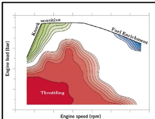
Limits of SI engine efficiency – Gasoline
