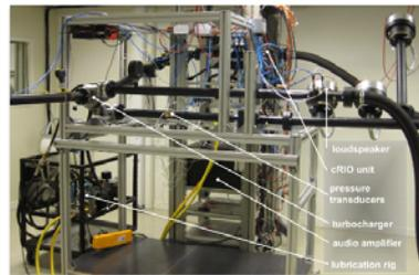
The TC acoustic characterization facility at KTH CCGEx (See the photo) have been used to determine accurate acoustical scattering and source data (full two-port data) at realistic operating conditions.
