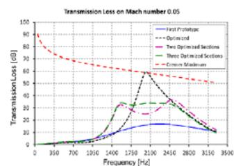
Sound transmission loss spectra from the optimization of the compact silencer prototype. The optimization technique is based on so called Cremer optimal acoustic impedance concept.
