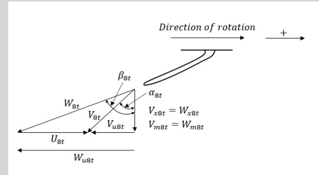
Outlet velocity triangle turbine rotor
