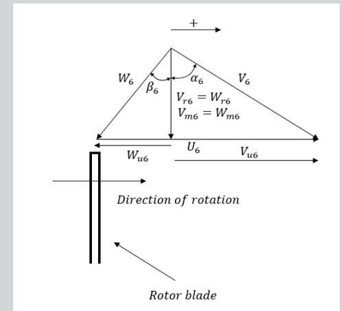
Inlet velocity triangle turbine rotor
