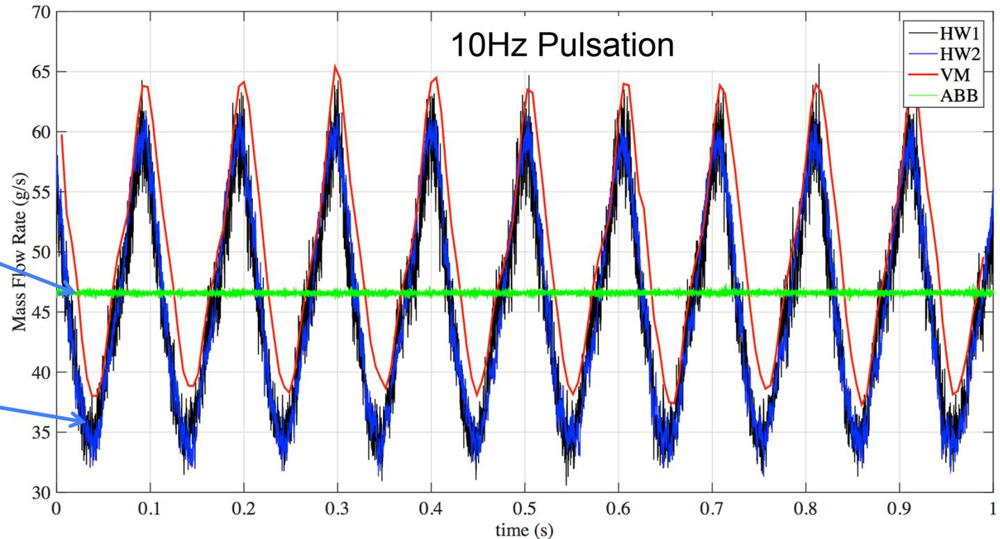
Work to be published: "Development of a Pressure Based Vortex-Shedding Meter: Measuring Unsteady Mass-Flow in Variable Density Fluids" (Meas. Sci. Tech.)
