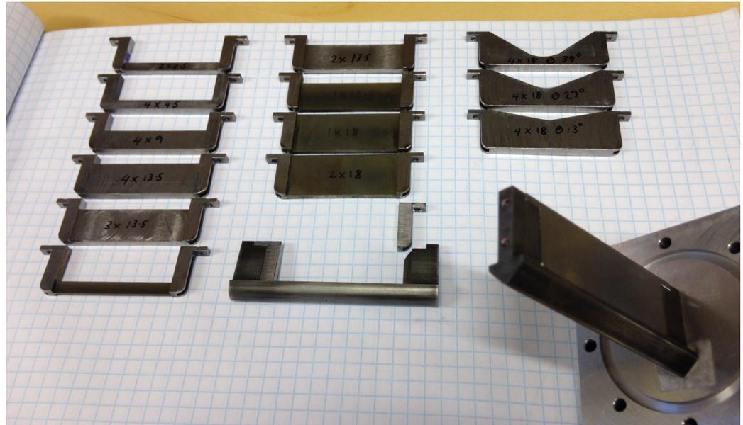
Examples of tail geometries and two fore-body design
