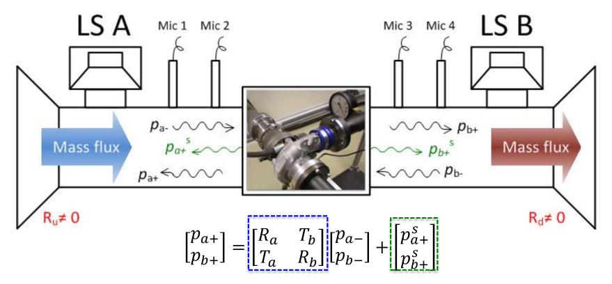
The acoustical performance of a flow duct element is determined by the full 2-port model which consists both the passive and the active parts.
