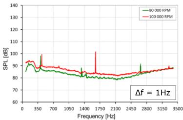
Inlet Sound Generation at Peak Efficiency Line
