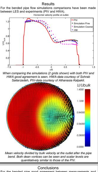
For the bended pipe good agreement between measurements and simulations can be shown for the outlet velocity profile. For the bended pipe simulations the software is predicting the flow accurately compared to experiments.
