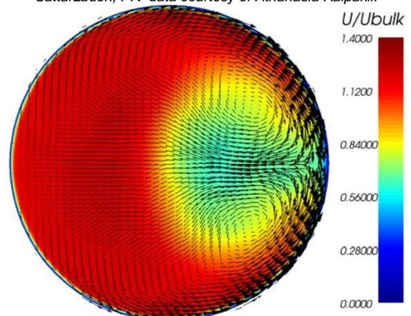
Mean velocity divided by bulk velocity at the outlet after the pipe bend. Both dean vortices can be seen and scalar levels are quantitatively similar to those of the PIV.
