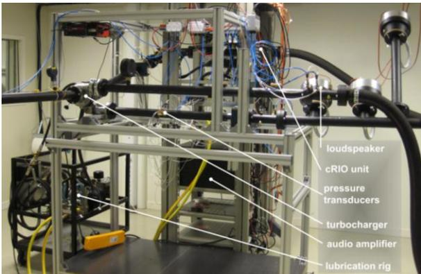
KTH CCGEX turbocharger test facility.
